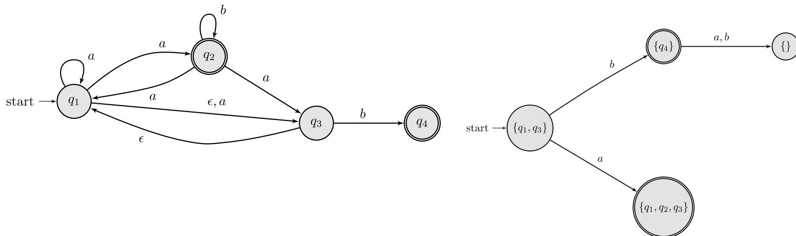
For inputs a and b we find all reachable states (via input+epsilon state) that start from  $q_4$ :
